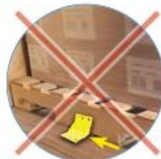
Pallet restraining devices that penetrate trailer flooring are NOT ALLOWED
