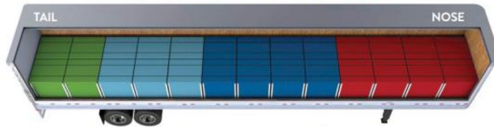
PO pallet trailer configuration (colors represent different POs)
