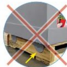
Stapling or gluing is NOT ALLOWED
