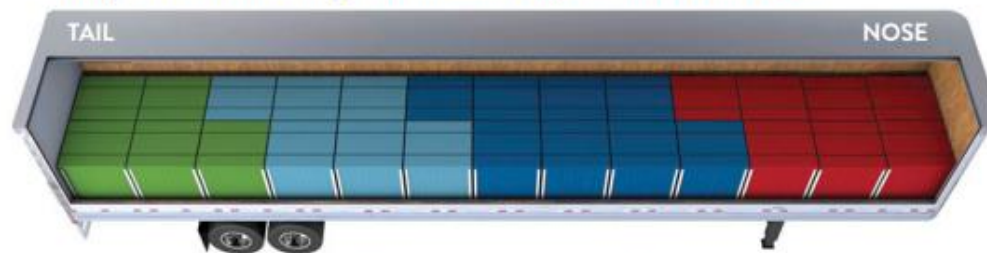
Item pallet trailer configuration (colors represent different POs)
